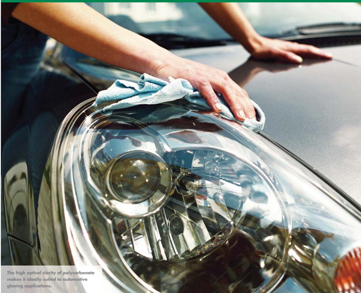
The high optical clarity of polycarbonate makes it ideally suited to automotive glazing applications.
